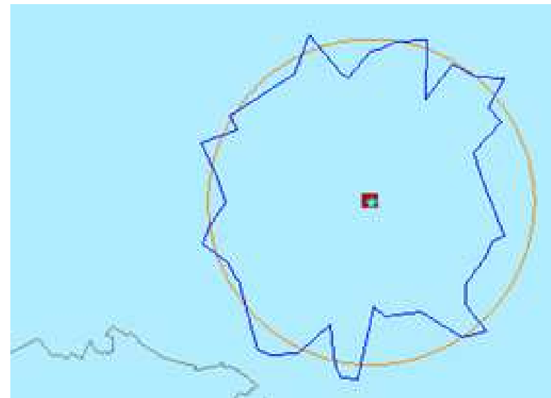
The above compares Squiggly (blue) with a concentric ring (orange – 1,210 m radius) at the 1,700 m SHDSL distance around Castle Hill exchange, Sydney)
